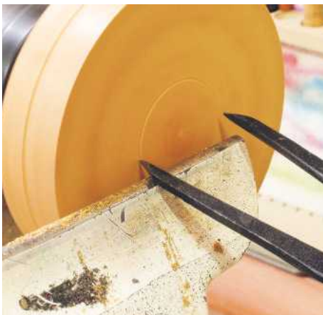
▲ Pic.7 Les is marking the diameter of the chucking recess on the bottom. The left-hand point makes a scratch that will line up with the mark on the right when correctly aligned
